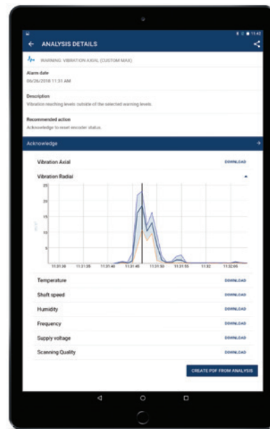
Quick report handling – For every serious deviation that occurs, the encoder automatically stores a fault buffer containing detailed data from both before and after the event. Warning reports and customized analysis reports are very easily to export as pdf and send to any recipient.
