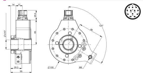
Model CHI 703/733 with tether arm and 12 pin M23 connector
