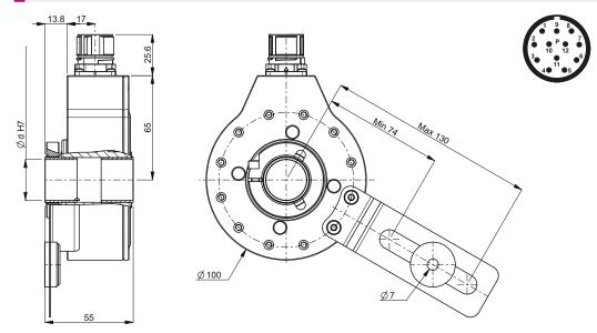
Model CHI 703/733 with torque bracket and cable
