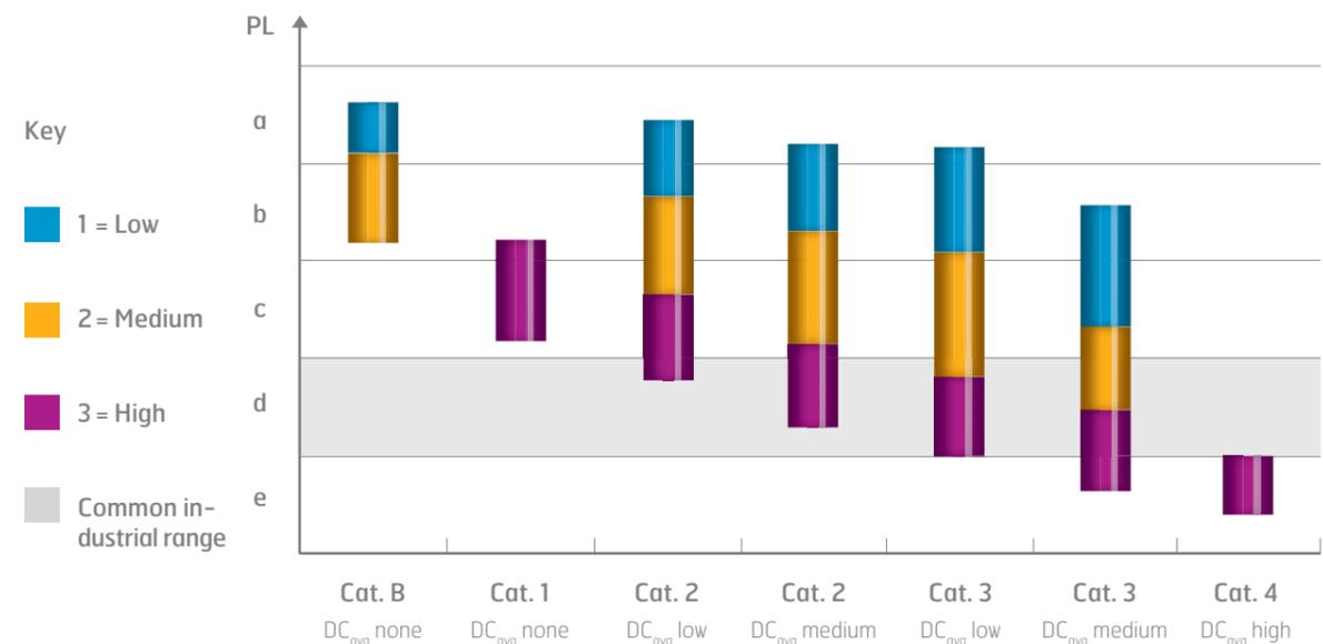
After finding out the required performance level for the application, use the examples on pages 8-9 to understand how the encoders meet the level in question. Depending on the design of the functional safety system, it is possible to achieve different performance levels.
